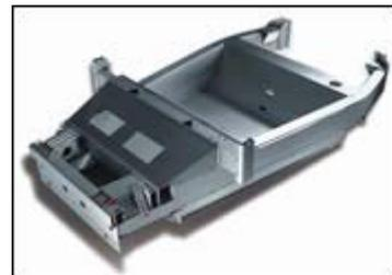
The shape of things to come? Lotus is bringing the aluminum bonding methods it pioneered with the Elise chassis to higher volume production. The first of the new vehicles are scheduled to be produced at the end of 2005.
